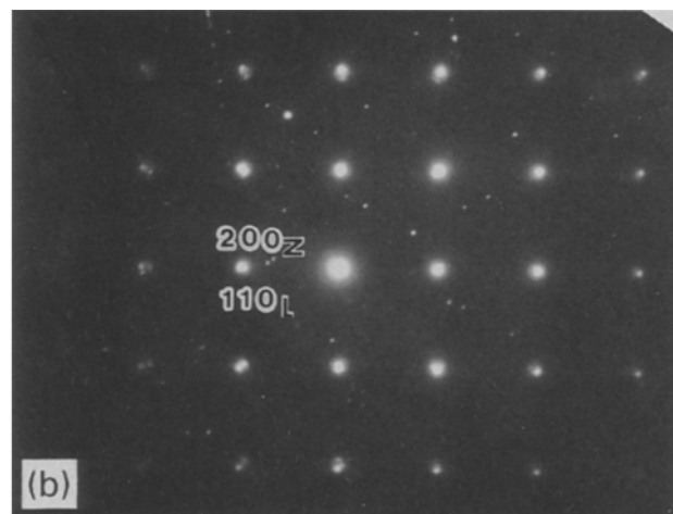
Figure 4 (a) Electron micrograph and (b) electron diffraction pattern taken from section parallel to interface between \text{La}_2\text{NiO}_4 and (001) cubic \text{ZrO}_2 after annealing at a temperature of 1173 K for 86.4 ks.
