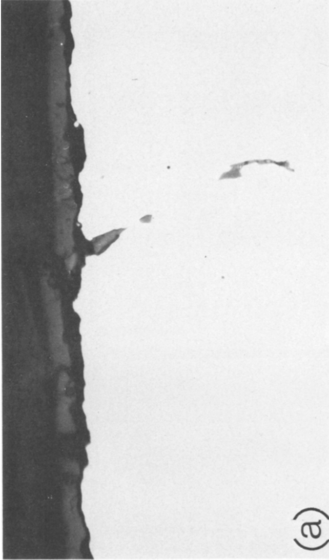
Fig. 18. Scales formed on Co-15Cr-8Al-1Y. (a) Cross section of sample oxidized 1000 hr at 1200°C ( \times 750 ); (b) surface of sample oxidized 1000 hr at 1100°C ( \times 200 ); (c) surface of sample oxidized 120 hr at 1200°C ( \times 200 ).
