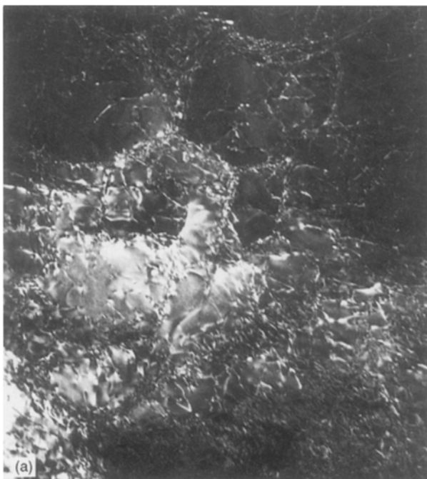
Figure 3 TEM micrographs of the as-quenched SiCw/6061Al composite: (a) dark field image and (b) bright field image.
