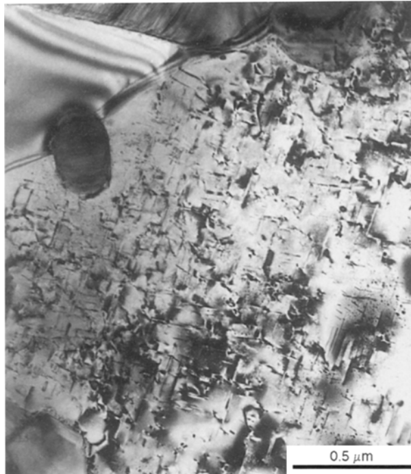
Figure 4 TEM micrograph of the composite aged at 170 °C for 10 min.
