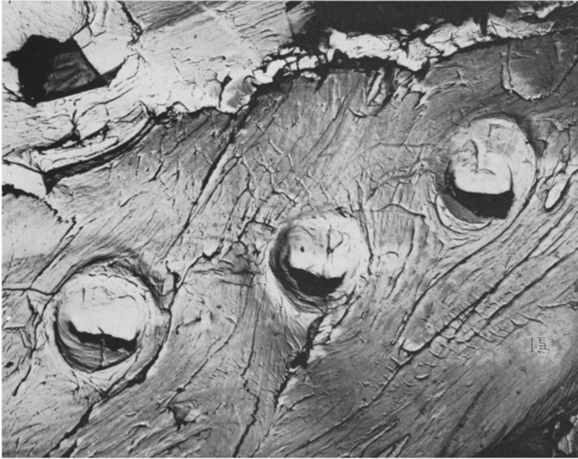
Fig. 4. Sample of fiber wall of Fagus sylvatica not heat treated. Presence of cracks here and in Figure 3 indicate that the cracks are due to preparatory techniques and are not induced by heat treatment. Approximately 2500:1.
