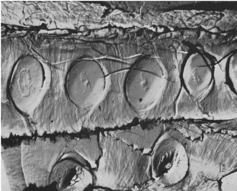
Fig. 3. Sample of fiber wall of Fagus sylvatica after heat treatment at 210 °C. Approximately 4 400:1.
