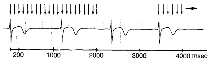
Fig. 1. ECG-gated FLASH sequence for detection of signal changes in the cardiac cycle. The same slice is excited 20 times perpendicular to the expected flow, starting every second or third R wave of the ECG
