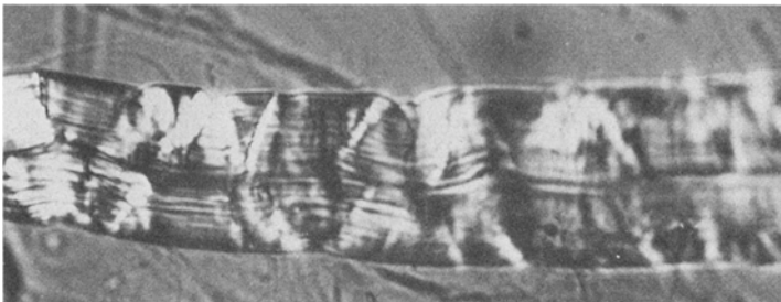
Fig. 1. Longitudinal delaminations in fibre walls
