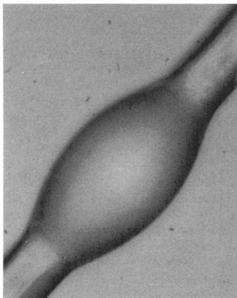
Figure 7 Drop of epoxy resin on a plasma-treated Spectra filament.
