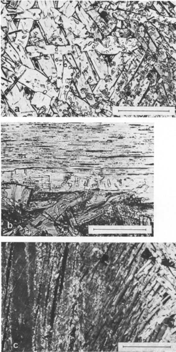
Fig. 3. Central, wholly recrystallised region near the centre of the specimen RH1. Most of the coarse grains are oriented NE-SW or NW-SE. The small equidimensional grains are also phlogopite, and the prismatic needles on the right hand side are forsterite. Plane polarised light. Scale bar is 200 \mu\text{m} . b Photomicrograph showing the gradation from deformed crystal displaying only KBB migration (on left) to completely recrystallised material (on extreme right). Note that many of the coarse new grains are subparallel to the host orientation. The specimen axis is horizontal, and the temperature increases from left to right. Crossed nicols parallel to plate edges. Scale bar is 500 \mu\text{m} . c Optically "clearer" strip along the margin of a specimen is outlined. It contains new grains up to 40 \mu\text{m} long, whereas the material above it is unrecrystallised. The coarsely recrystallised material below the cleared strip is the reaction rim between the specimen and the talc jacket. Plane polarised light. Scale bar is 80 \mu\text{m} .
