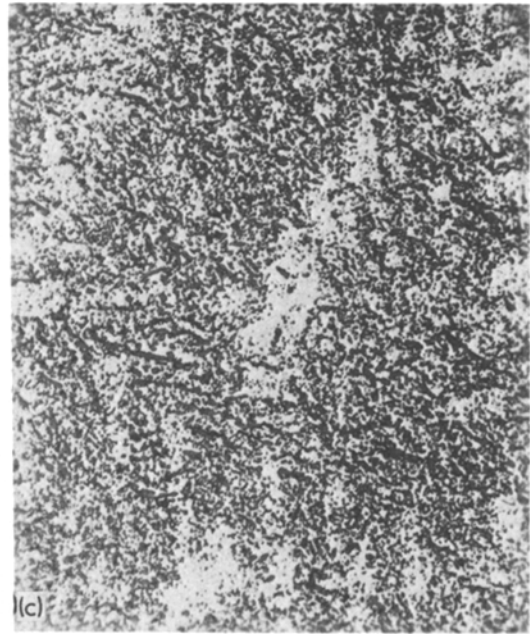
Figure 5 Optical micrographs of Al-Si eutectic alloys showing the effect of annealing on the silicon morphology of the chill-cast alloy ( \times 488 ). (a) Chill-cast. (b) Annealed, 350^\circ\text{C} , 1 h. (c) Annealed, 500^\circ\text{C} , 1 h.
