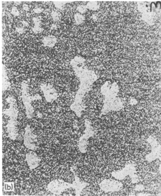
Figure 5 Optical micrographs of Al-Si eutectic alloys showing the effect of annealing on the silicon morphology of the chill-cast alloy ( \times 488 ). (a) Chill-cast. (b) Annealed, 350^\circ\text{C} , 1 h. (c) Annealed, 500^\circ\text{C} , 1 h.
