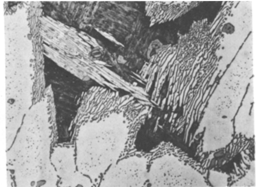
Figure 7 Alloy slowly cooled from 1000 to 725° C and quenched, showing fine \kappa_{IV} precipitation within the \alpha grains ( \times 480 ).
