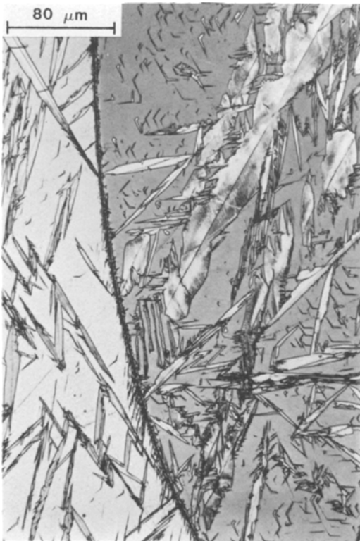
Figure 4 Light micrograph of a 1.84% C sample brine-quenched from 1150°C. This was taken very near the centre of the specimen. Note the reaction product at the austenite grain boundary.
