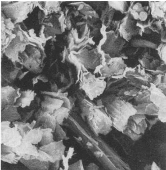
Figure 3 SEM of diamond saw cut carbon-carbon composite cross-section (Thornel 75S/FF-26 after third graphitization), \times 5200 .
