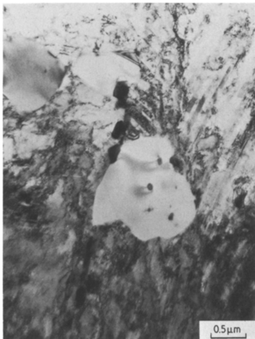
Figure 16 316 steel isothermally annealed at 800° C for 15 minutes which was subjected to a tensile pre-strain of 40%.
