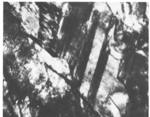
Figure 11 Microstructure of a tensile specimen given 3% total elongation at room temperature (bright-field images).
