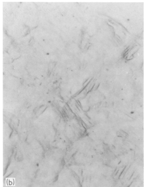
Figure 3 Optical micrographs showing surface relief effects associated with stress-induced growth and/or re-orientation of the most favourably oriented existing martensite. (a) 1%, (b) 2%, and (c) 3% total elongation at room temperature.
