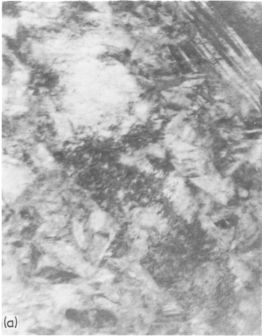
Figure 10 Microstructure of a tensile specimen given 8% total elongation at room temperature, (a) Bright-field image, and (b) dark-field image.
