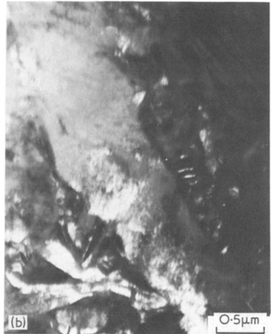
Figure 10 Microstructure of a tensile specimen given 8% total elongation at room temperature, (a) Bright-field image, and (b) dark-field image.
