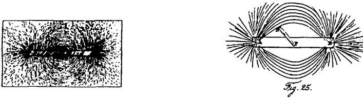
Figure 2. (a) Actual pattern of lines of force surrounding a bar magnet (from Faraday (1839–55), vol. 3); (b) Schematic representation of lines of force surrounding a bar magnet.
