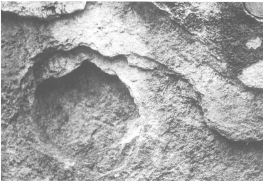
Fig. 3. (a) An example of sandstone damage: the black surface crust (layer A ) is clearly shown; where exfoliation occurs, the underlying powdered layer ( B ) is lost within a short time, exposing the undamaged rock to a new cycle of chemical weathering. (b) The decayed sandstone surface shows exfoliation revealing concentric cracks which have been produced by dissolution of the calcium carbonate, the soluble portion of the rock.
