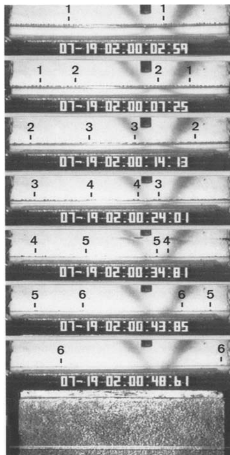
Fig. 13. Determination of the true strain rate by the 'particle tracking method'. The distances of the same two particles i-i are measured at two different instants of the deformation and reveal the strain rates given in the last column of Table 2. Material: Low density polyethylene (Lupolen 1810 H of BASF, Charge 681133259). Test conditions: Temperature 150 ^{\circ}\text{C} , nominal strain rate 0.1 \text{s}^{-1}
