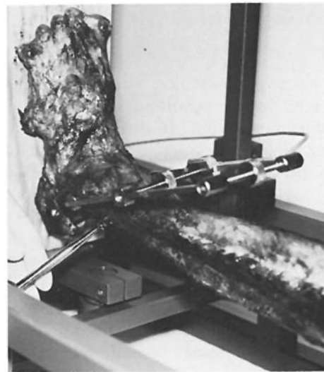
Fig. 3. a This device was used to get a constant compression force between the two malleoli when inserting the syndesmotic screw. The two arms of the device could be compressed by turning the screws. Strain gauges were glued to one arm and the compression force could be recorded using a voltmeter. b The device is attached to the specimen while the syndesmotic screw is being inserted
