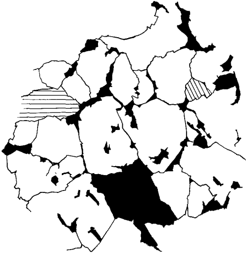
Fig. 19. Granodiorite, Sunday Pluton, Washington. Quartz synneusis patterns. Corroded aspect of quartz grains emphasized by surrounding orthoclase. Width 9.1 mm
