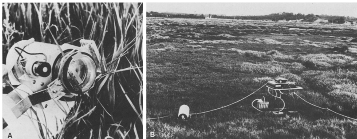
Fig. 2. (A) View of the porometer supported on a clamp with a blade of Spartina maritima inserted into the cuvette between foam rings. The small sensor next to the cuvette lid measures photosynthetically active radiation. (B) The porometer instrumentation as used during measurements in the salt marsh near Corroios. The measurement cuvette is protected in a small basket; a polypropylene container is used to buffer CO 2 partial pressure changes of the ambient air entering in the line from the left; power is supplied from a generator via the cable at the right; and the pumps, gas analyzer, recorder, and digital read-out units are supported on the small table
