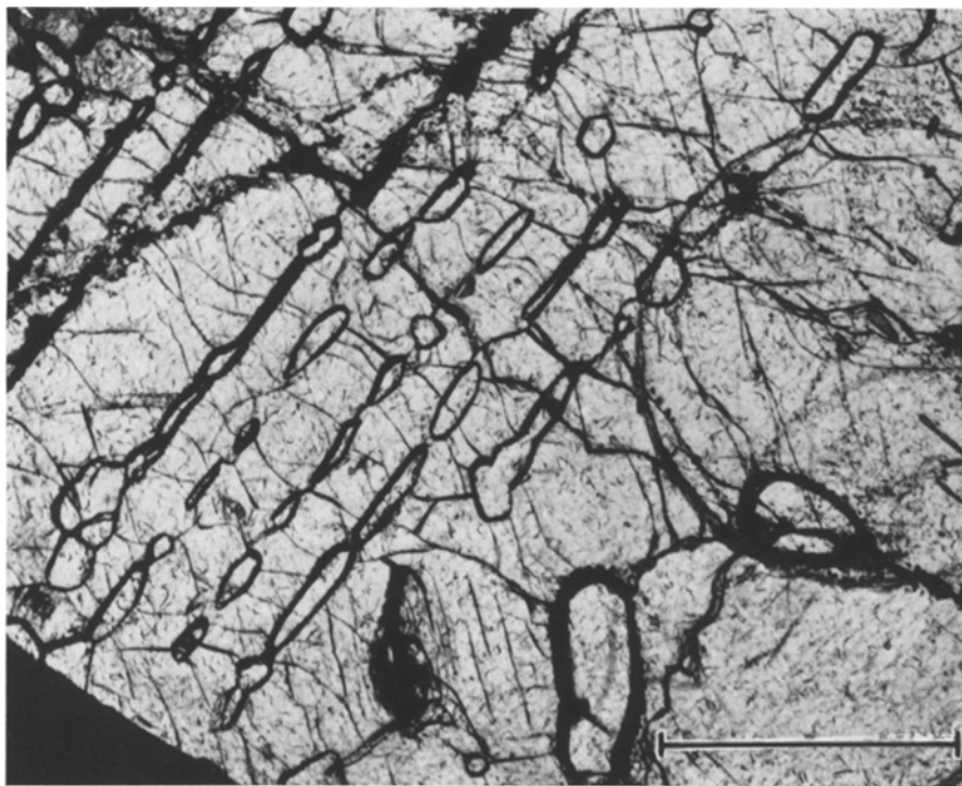
Fig. 6. Photomicrograph of part of a large clinopyroxene crystal in the spinel pyroxenite (R394) showing strings of garnet blebs (apparently exsolved) parallel to (100). Within the inscribed circle are several spindle-shaped spinels oriented parallel to (010) i.e. perpendicular to the garnet strings. The spinels are distinguished from the garnets by their small size, grey colour and lack of dark rims. The largest spinel in the centre of the circle was analysed on the electron probe. Scale \frac{1}{2} mm
