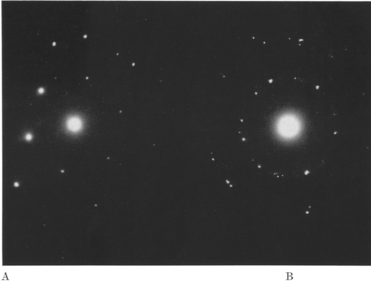
Fig. 3. Electron diffraction patterns obtained from two graphite crystallites in sample 23678 (fully ordered graphite). Several other diffraction patterns were obtained from particles in this sample; all were closely similar. Patterns represent a portion of the graphite lattice; visible lattice points are 100 and 110 (002 lattice points visible on some other patterns). Figure B produced by more than one superimposed co-planar crystallites
