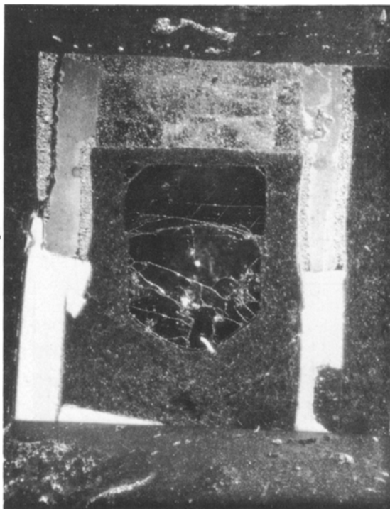
Fig. 2. An example of a "successful" pyrope-almandine couple, which preserved the (horizontal) interface after a run at 38 Kbar, 1,475° C, 26.7 h (Run # 16). Although the garnets were partly fractured, most of the interface was preserved intact. The interface is indicated by horizontal lines on the sides of the couple. The sectional width of the couple is 0.25 cm
