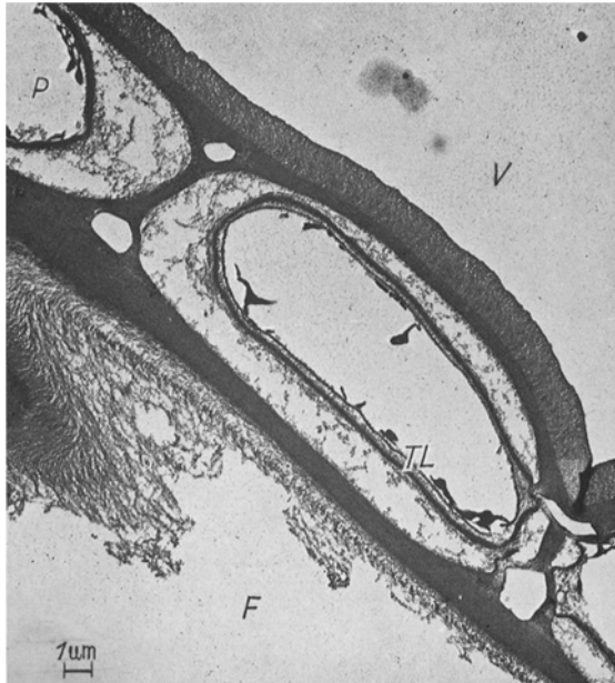
Fig. 13. Tangential section of aspen tension wood. The secondary wall of the two parenchyma (P) cells contain very little lignin and possess a terminal lamella (TL) and a warty layer.
