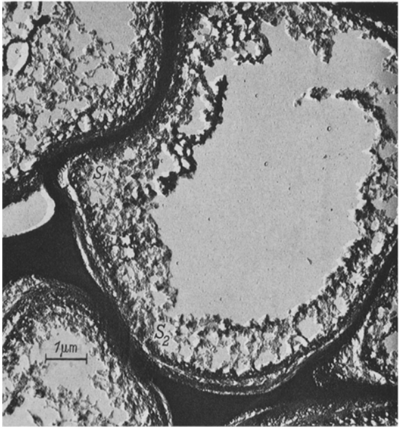
Fig. 2. Transverse section of three fibers of normal beech wood. The lignin meshwork in S 2 is partly disrupted.
