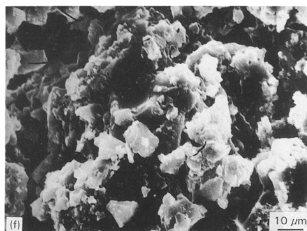
Figure 4 Scanning electron micrographs of SiC synthesized from (a) TEOS + phenolic resin, (b) MTES + phenolic resin, (c) copolymer + phenolic resin, (d) TEOS + ethylcellulose, (e) MTES + ethylcellulose, (f) TEOS + PAN, (g) TEOS + starch.
