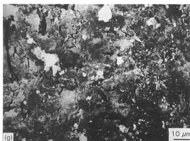
Figure 4 Scanning electron micrographs of SiC synthesized from (a) TEOS + phenolic resin, (b) MTES + phenolic resin, (c) copolymer + phenolic resin, (d) TEOS + ethylcellulose, (e) MTES + ethylcellulose, (f) TEOS + PAN, (g) TEOS + starch.
