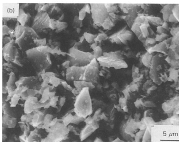
Figure 2 SEM micrographs of an Al 2 O 3 particle cluster (without any binder).
