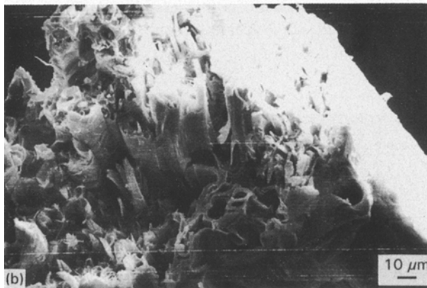
Figure 10 Magnified view of 3-year-old plant fibre fractured at 30°C.
