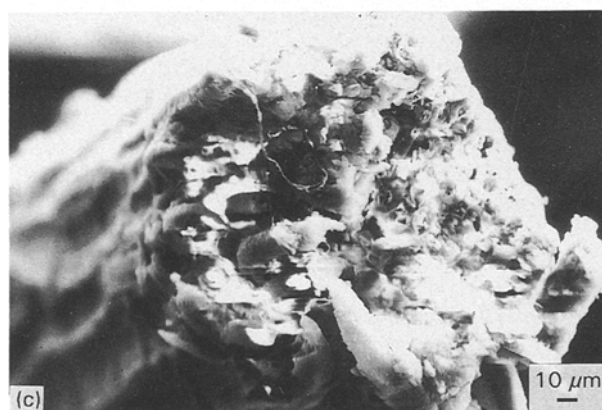
Figure 7 SEM fractograph of 5-year-old plant fibre fractured at (a) 30 °C, (b) 80 °C, (c) 100 °C.
