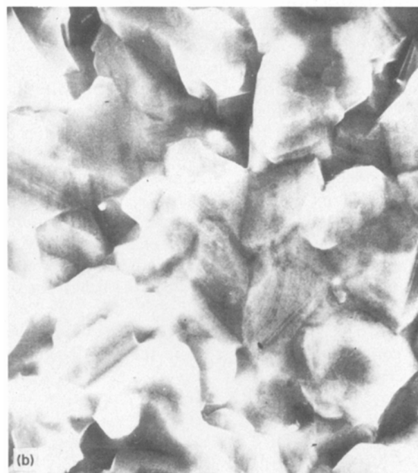
Figure 3 The W morphology after cofiring (1850 °C, 2 h): (a) No. 2 paste, and (b) No. 5 paste (see Table I).
