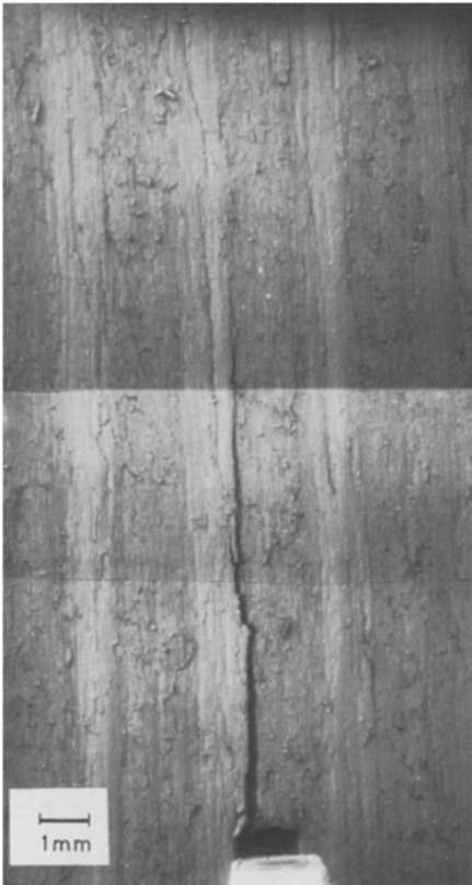
Fig. 12. Crack induced in the first stage of loading in a specimen with the grain parallel to the notch
