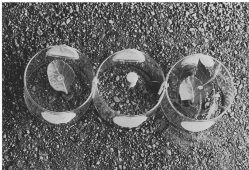
Fig. 4. Choice chamber placed over test plants. One collard leaf is in the section at the left and one collard leaf and two tomato leaves are in the section at the right
