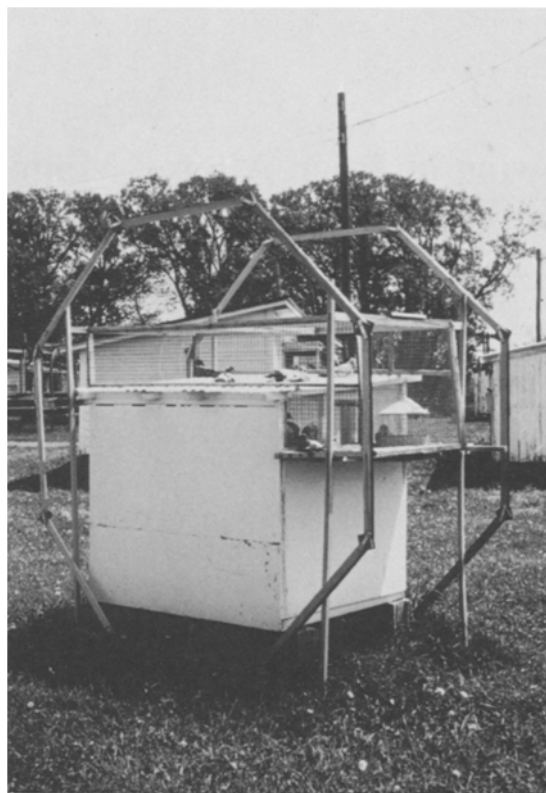
Fig. 1. The experimental loft within Helmholtz coils; the inhabitants could see the sun only in altered relationship to the magnetic field
