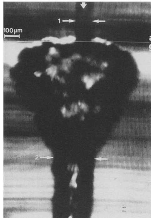
Fig. 5. The shape of the laser drilled hole in an agar-gelatin target at the end of the laser pulse. The hole diameter at the position 1 indicates the normal diameter drilling into the rigid agar material. Just below the material boundary the diameter increases up to more than 3 times than the one 1 mm below (position 2). (CO 2 laser: 300 J/cm 2 , \tau = 400 \mu\text{s} )
