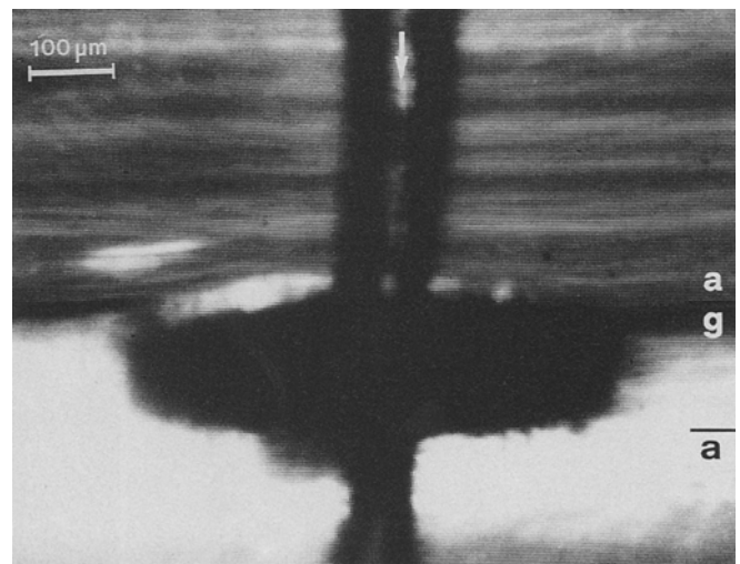
Fig. 6. The picture shows the shape of the hole at the end of the CO 2 laser pulse drilled into the composite structure of an agar-gelatin-agar target used to simulate the layer structure of skin. Inside the gelatin layer the hole diameter is about five times larger than in the agar material. (CO 2 laser: 300 J/cm 2 , \tau = 400 \mu\text{s} )
