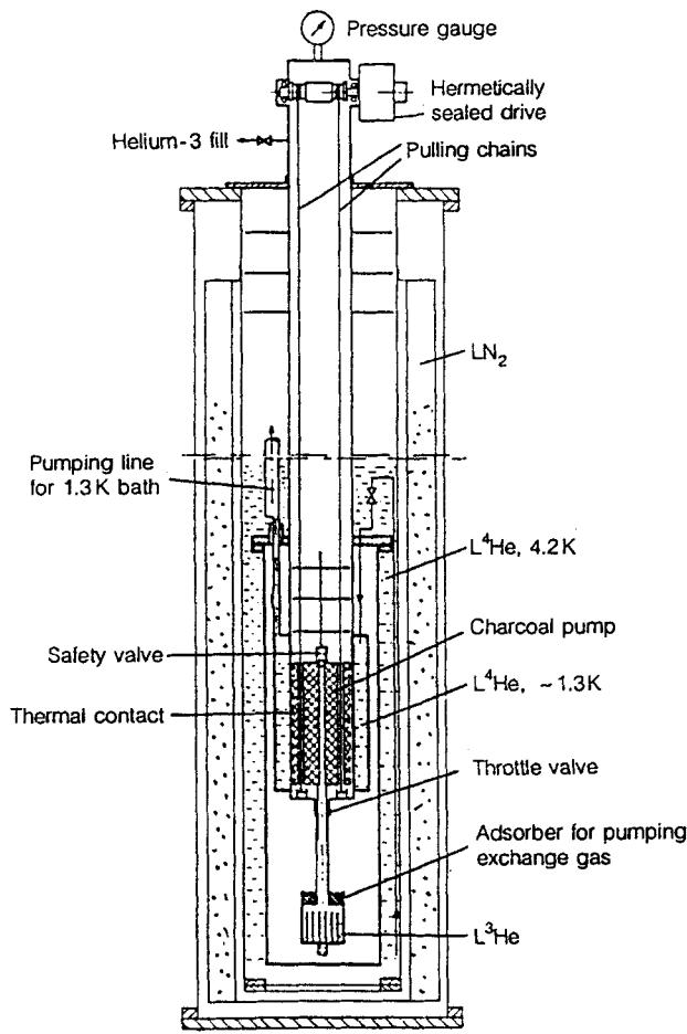
Hermetically sealed, charcoal pumped  ${}^3\text{He}$  refrigerator. The charcoal pump can be raised or lowered by means of a chain drive operated via a hermetically closed rotating seal
