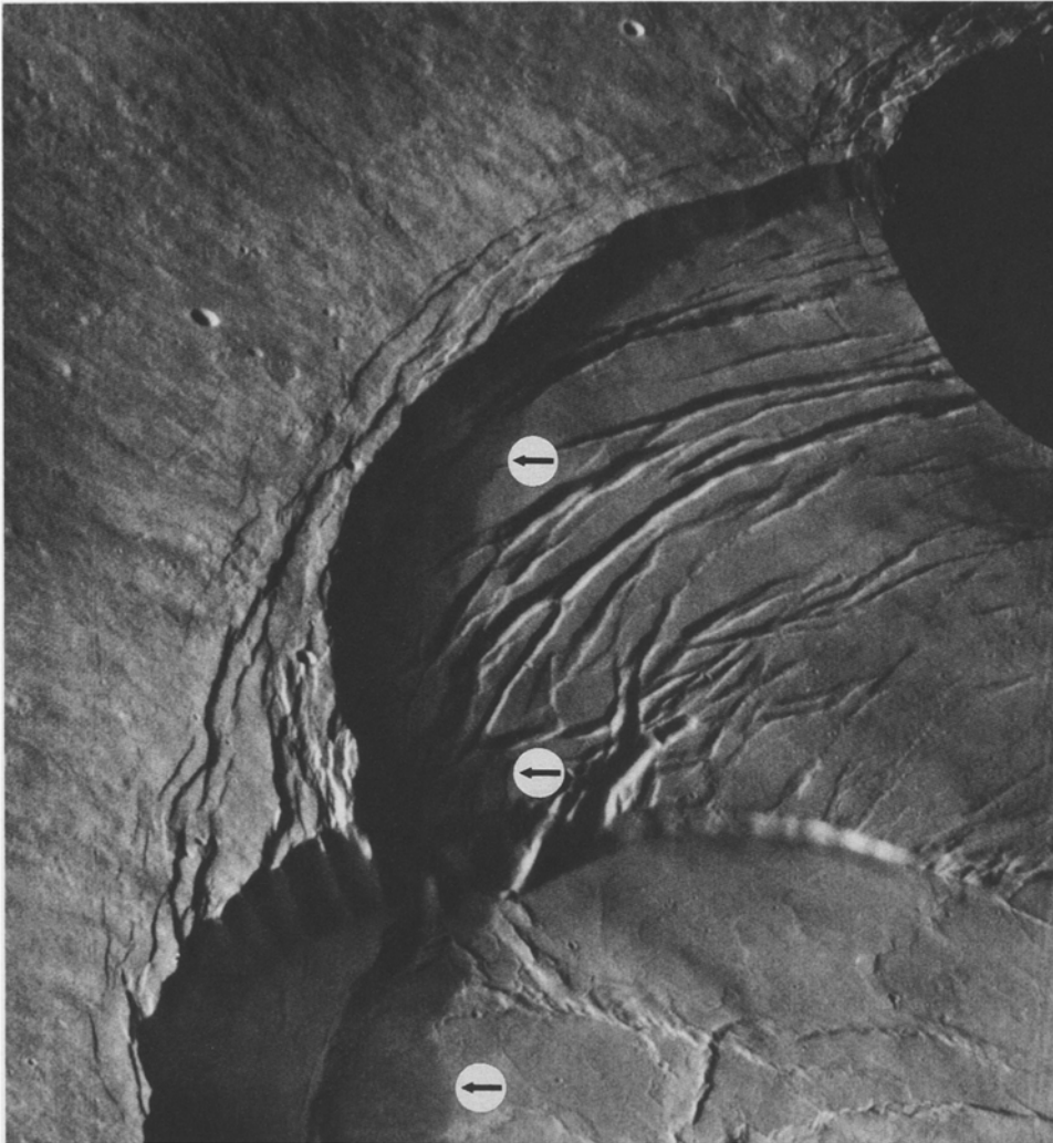
Fig. 4. Oblique view of the western side of the Olympus Mons summit caldera, showing the location of shadows ( arrowed ) on the caldera floor. Knowledge of the illumination geometry and the pixel resolution permit the height of the caldera wall to be calculated from data such as these. Note that image data from which the shadow measurements were derived have a spatial resolution of 28 m/pixel on the western side of the caldera, and data for the eastern side have a resolution of 160 m/pixel. See Fig. 2a for location. Viking Orbiter image 475S03 (INA = 80°)
