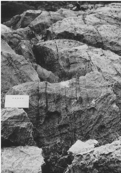
Fig. 3. Field photograph of steeply inclined (towards north) chrome-spinel seams within unit 1 rocks [Ordnance Survey Grid Reference (NG 4787 1967)]. Scale bar on notebook is in centimetres
