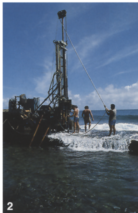
Fig. 1. Drilling on the barrier reef of Tikehau Atoll (Tuamotu) (December 1988 to March 1989) by ORSTOM team led by Dr. F. Rougerie. Foreground 30-m-deep hole has been permanently fitted with a four channel polyethylene hose; sampling is by peristaltic pump with 100 ml/min flow rate. Dissolved nutrients O 2 , pH, salinity, alkalinity are measured in the ORSTOM facility on this atoll. Background Drilling of a second hole, 3.5 cm in diameter, closer to the outer algae-coral rim of the barrier reef. These operations are performed as a tentative validation of the geothermal endo-upwelling process and are financially supported by ORSTOM (TOA Department) and INSU/CNRS (France)
