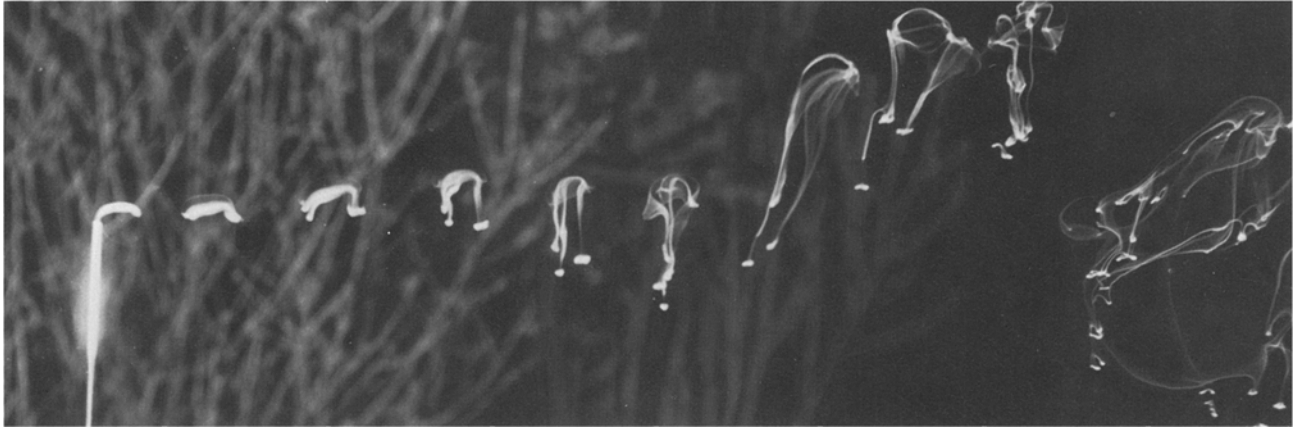
Fig. 8. Simulation of a temporally patterned chemical signal. Air laden with a visible marker (titanium tetrachloride) is pulsed at the rate of 2 'puffs'/s from the glass capillary shown at left (wind speed \cong 11 cm/s). The pulses evidently remain discrete over the distance (60 cm) spanned by the photograph
