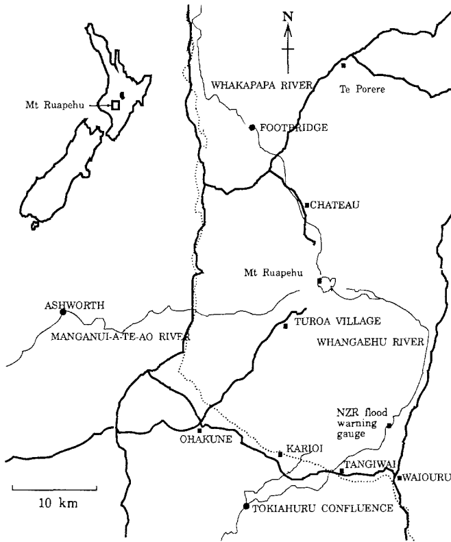
Fig. 1. Positions of lahar recording sites about Mt. Ruapehu. The dotted line denotes the main railway line north, the heavy lines are main roads about Mt. Ruapehu, and the thin lines are the main streams draining Mt. Ruapehu. Stage recorders are shown as solid circles at the Tokiahuru Confluence, the Whakapapa Footbridge, and at Ashworth on the Manganui-A-Te-Ao River
