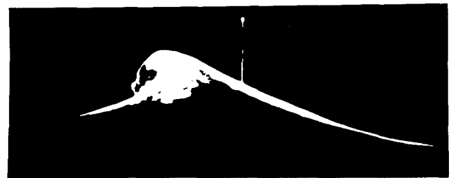
Fig. 3. Photograph of a plunging breaker observed in the water tank (from a 16 mm movie film)
