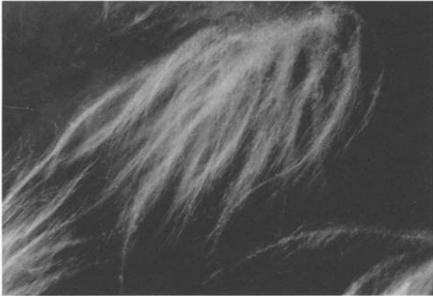
Fig. 3. Part of a disintegrated pellet after 65 h, \times 12
