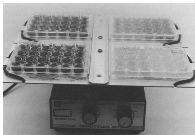
Fig.1: Photograph of transparent microtiter dishes used as a microtest system for photoautotrophic growth of Chenopodium rubrum cell suspensions; dishes are shown without lid
