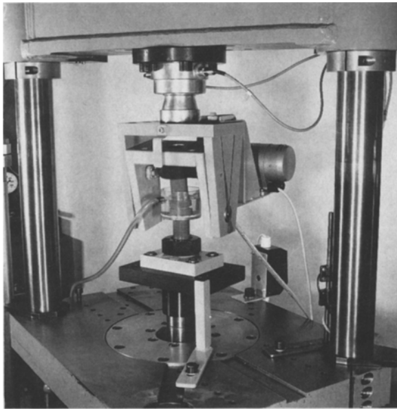
Fig. 3. Servohydraulic rig used for testing the prostheses. (Institute of Lightweight Construction, Dresden, GDR)
