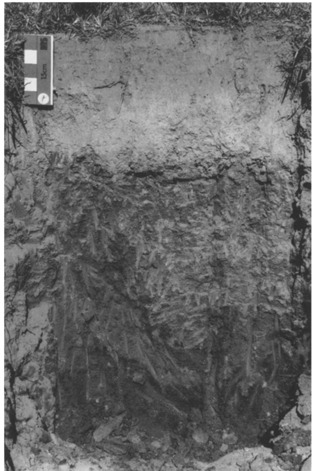
Fig. 1. Aeric Albaqualf profile illustrating basic physical concepts. The profile contains about 10% clay minerals to a depth of ~0.25 m, where they increase to ~30%. Silt and fine sand decrease correspondingly. The boundary between A1 and A2 horizons appears as colour change at ~0.12 m
