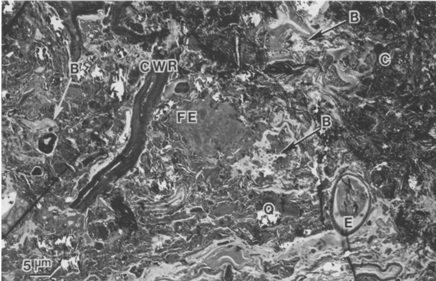
Fig. 1. General view of a clay. Small colonies of bacteria lie in small pores, and as isolated individuals throughout the fabric. G/Os/Pb. See footnote on p. 193 for explanation of symbols
