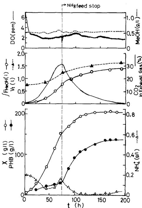
Fig. 5. Experimental results for mass production of PHB by fully automatic fed-batch culture. Ammonia feeding was stopped when the cell concentration reached 160 g/l at 75 h
