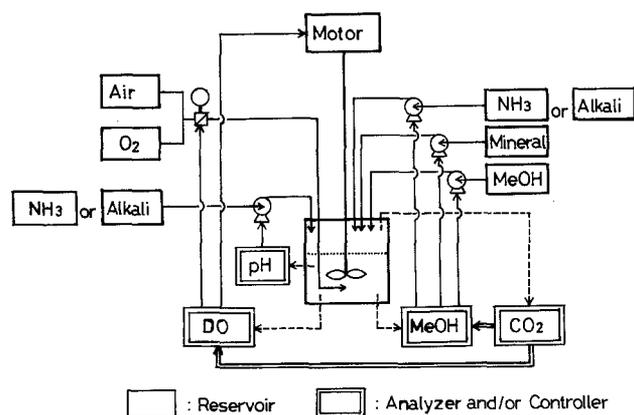
Fig. 1. System for computer-aided fed-batch culture
