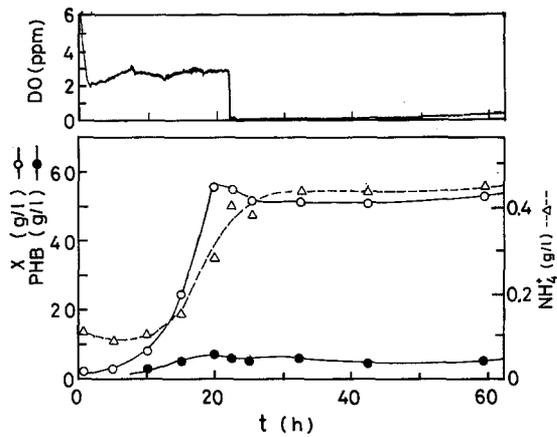
Fig. 7. Effect of DO on PHB formation. When the cell mass concentration reached 50 g/l, aeration condition was changed to let cells DO-deficient
