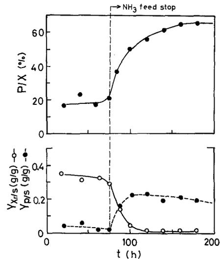
Fig. 6. Time courses of PHB content and correlation between the yield of PHB ( $Y_{P/S}$ ) and the yield of residual biomass ( $Y_{Xr/S}$ ) during the fully automatic fed-batch culture
