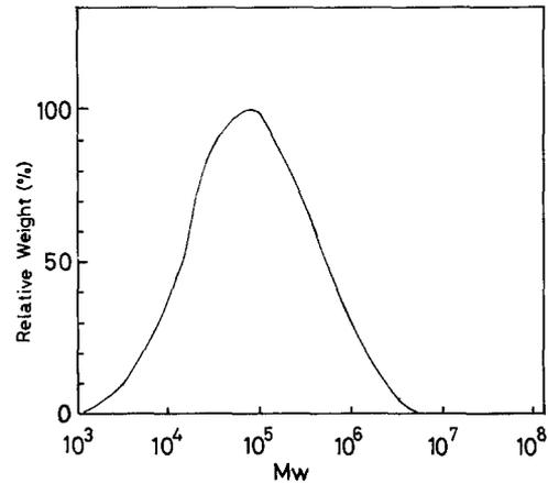
Fig. 8. Molecular weight distribution curve of the PHB produced by *Pseudomonas* sp. K
