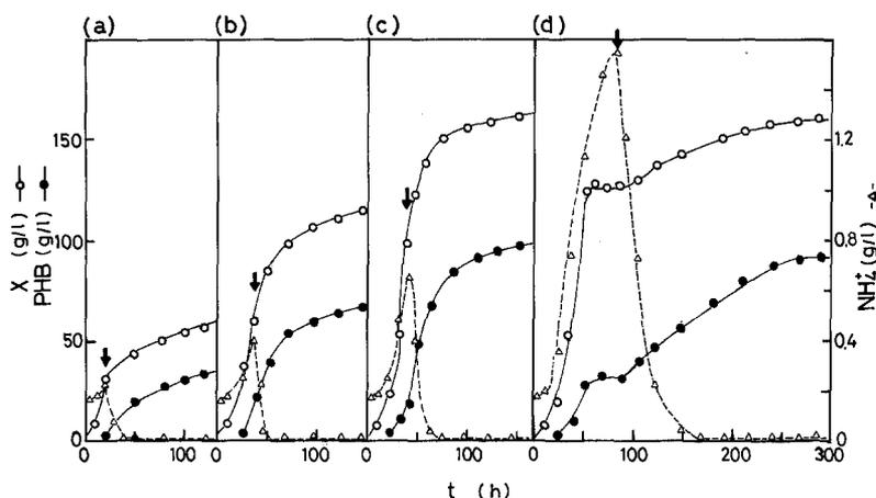
Fig. 3. Effect of ammonium deficiency at various culture phases on PHB formation. Ammonia feedings were stopped when the cell mass concentrations reached (a) 25, (b) 60, (c) 100, and (d) 130 g/l, as indicated by arrows
