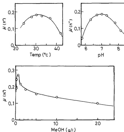
**Fig. 2.** Effects of temperature, pH, and methanol concentration on the specific growth rate of *Pseudomonas* sp. K grown on Medium C
