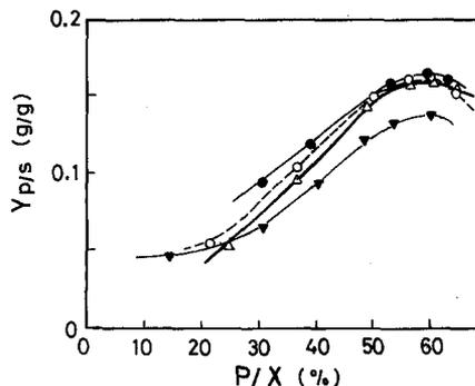
Fig. 4. Correlation between the PHB yield based on methanol consumed,  $Y_{P/S}$ , and PHB content. Ammonia feedings were stopped when the cell mass concentrations reached  $\bullet$ , 25;  $\circ$ , 60;  $\Delta$ , 100; and  $\blacktriangledown$ , 130 g/l
