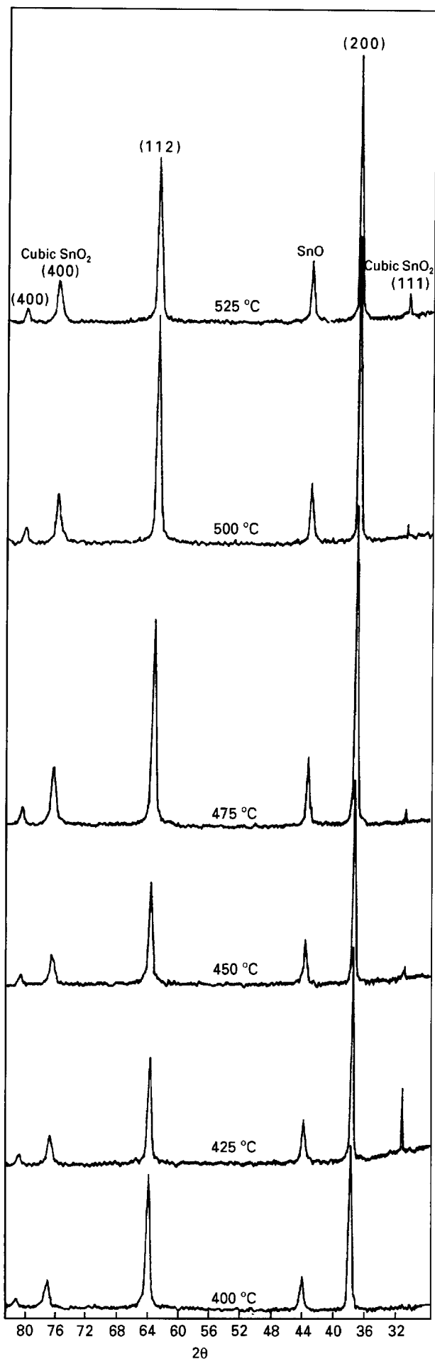
Figure 1 X-ray diffraction traces of \text{SnO}_2 films at different substrate temperatures.
