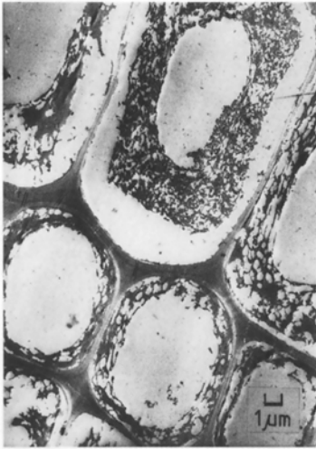
Fig. 9. Ancient pinewood ( Pinus massoniana ) from a submerged Chinese junk, 700 years old. TEM micrograph
