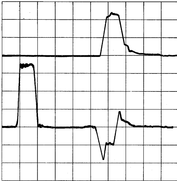
Figure 2. A typical recording of the incident, reflected (lower beam) and transmitted (upper beam) pulses, drawn from the oscilloscope image.
