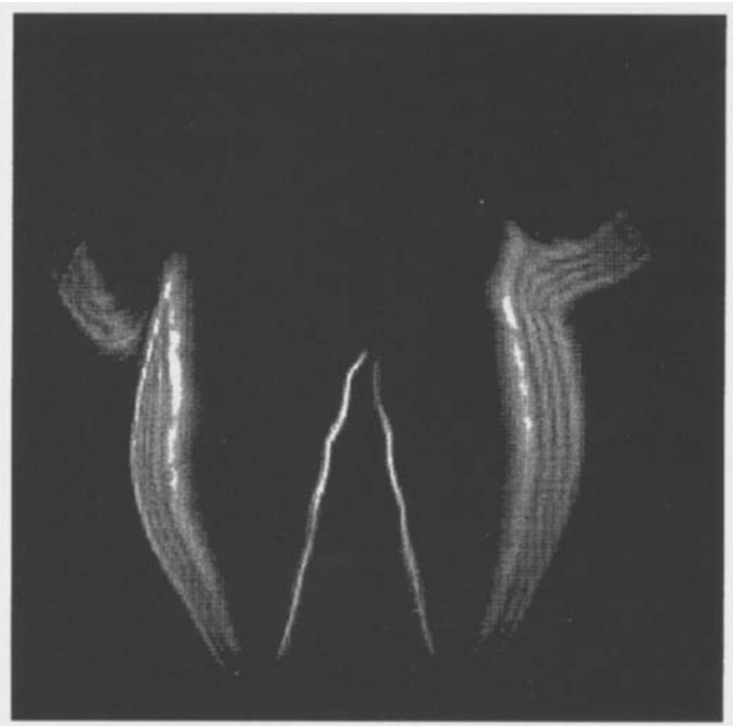
Fig. 3. Schlieren image of a +g laminar methane/air flame with flow rate of 0.42 liter/sec and \phi = 0.9
