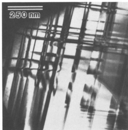
Fig. 11. A higher magnification \mathbf{g} = (1, \bar{1}, 0)^* satellite dark field image as for Figure 8a showing in greater detail the complicated contrast variation
